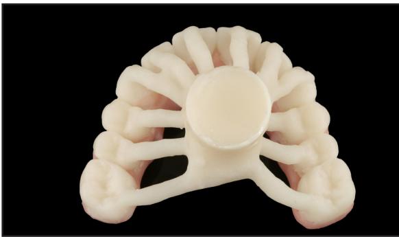
Fig. L Each tooth is connected by its own sprue when the white porcelain layer is pressed.
