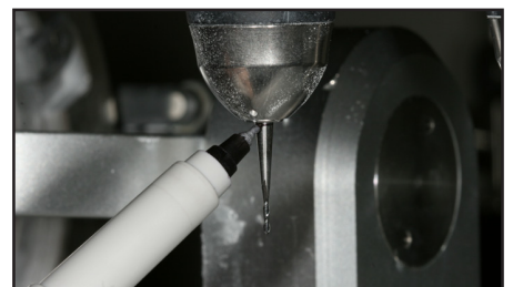
Fig. F For the "drop the pin" milling technique, the milling bur is dropped approximately 0.75mm...
